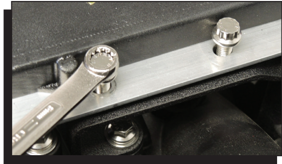
Figure 8 Tighten the Fuel Rail Bolts.
