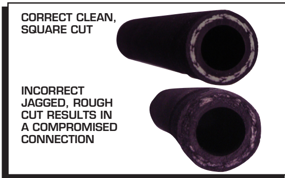
Figure 12 Severing the Hose Properly.
