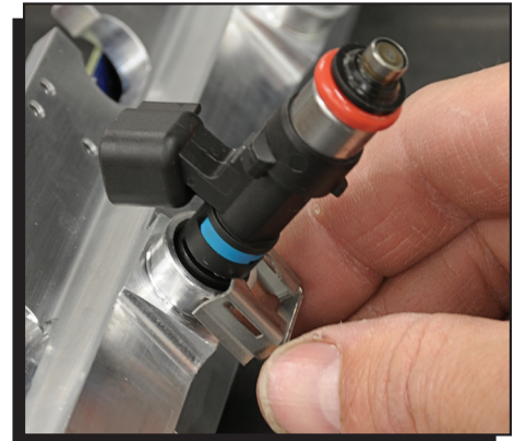
Figure 6 Installing the Injectors.
