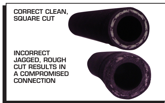
Figure 25 Severing the Hose Properly.
