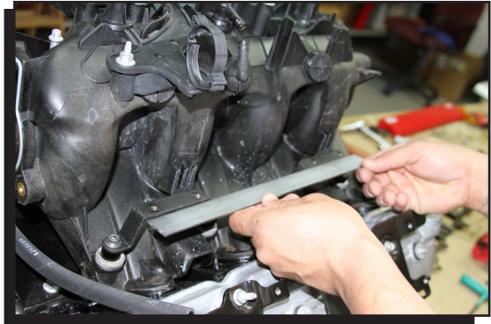
Figure 12 Straight Edge Check of Brackets.
