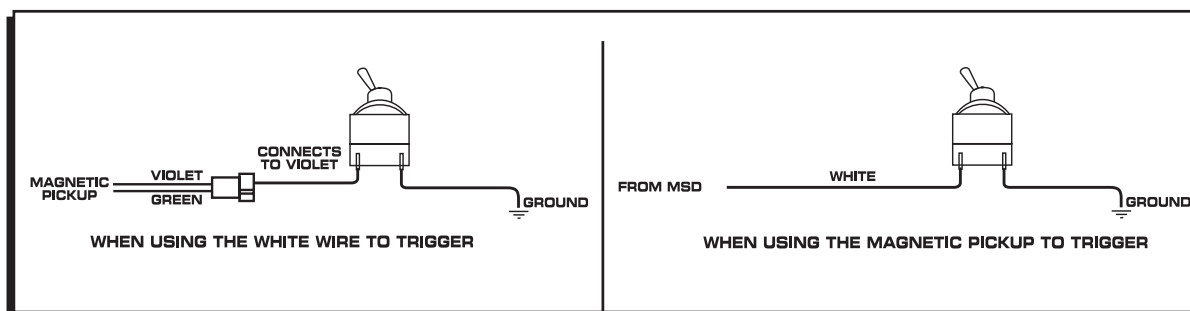
Figure 4 Connecting a Theft Deterrent Switch Through the MSD Ignition.
