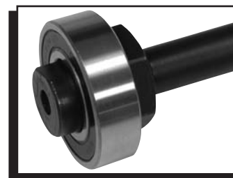
Figure 9 Installing the New Bearing.
