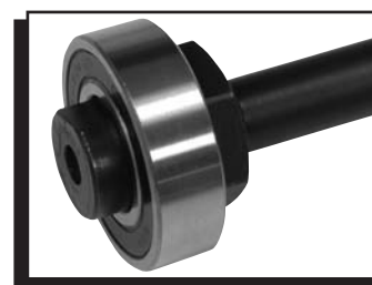
Figure 9 Installing the New Bearing.
