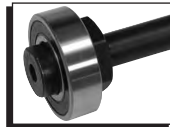
Figure 7 Installing the New Bearing.
