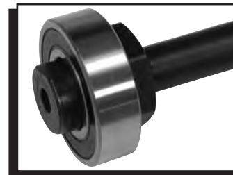
Figure 7 Installing the New Bearing.
