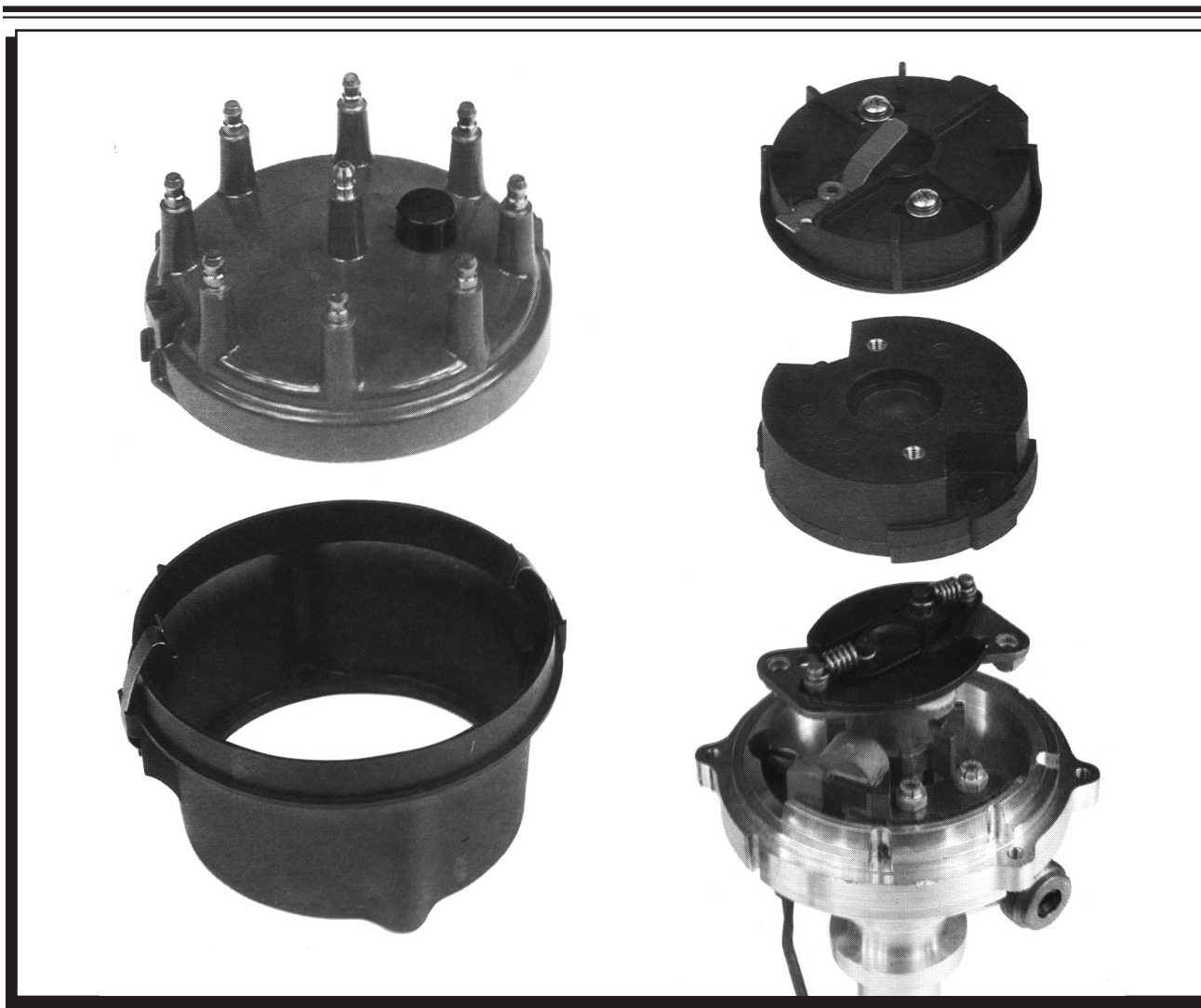
Figure 3 Installing the Cap-A-Dapt.
