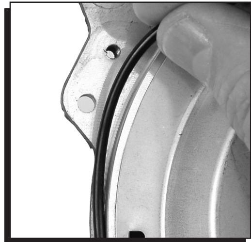
Figure 2 Installing the Distributor-to-Isolator Seal.
