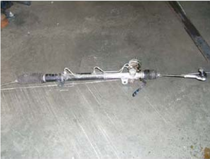
Pic. 3. Steering rack removed
