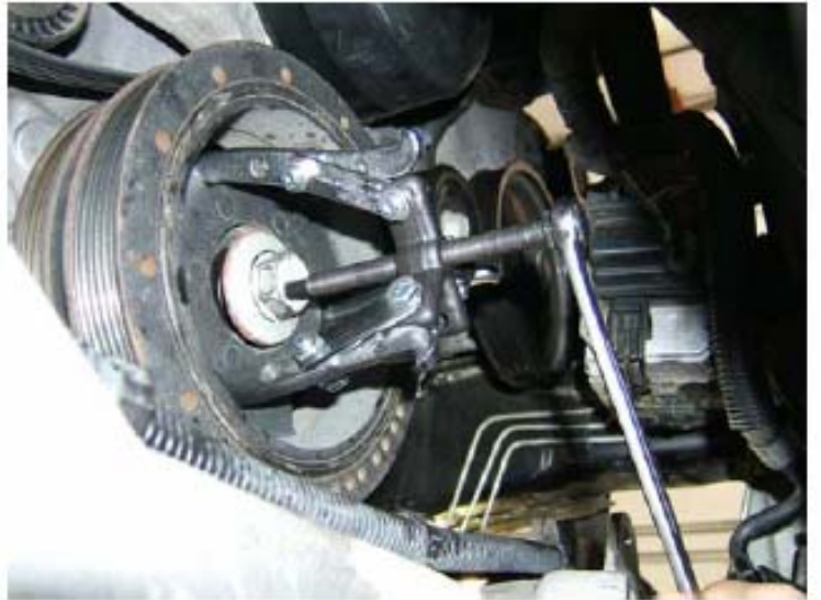
Pic. 4 Using the puller tool
