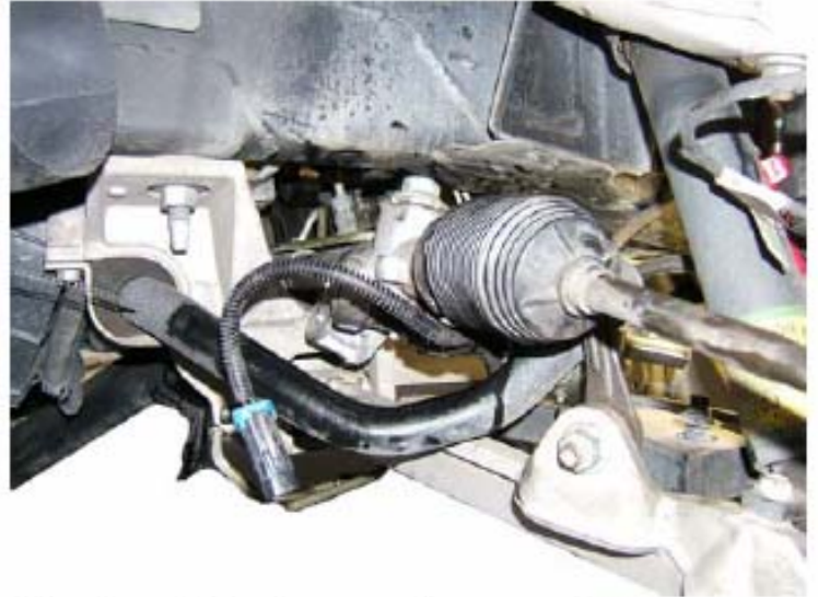
Pic. 2 Steering rack removal
