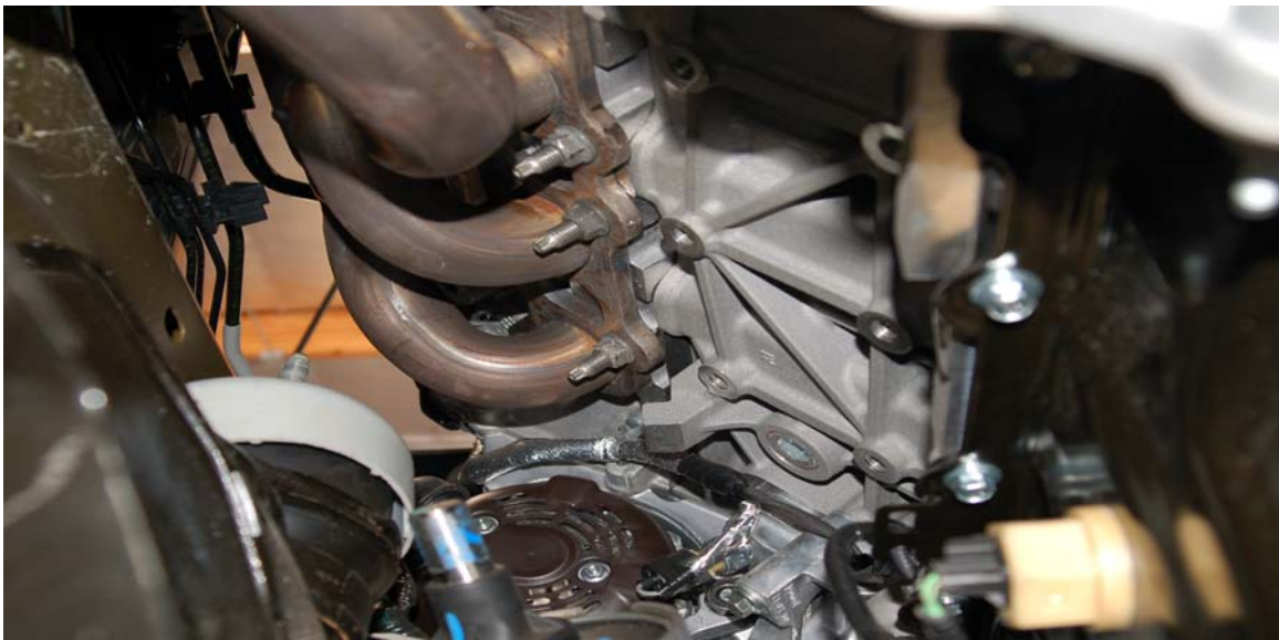
Fig 1. Motor Mount removed. Shows nut access.
