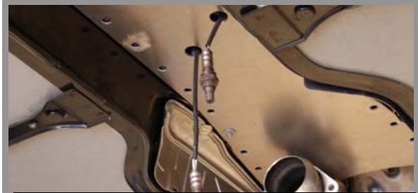
C6 Oxygen Sensor Holes Shown
