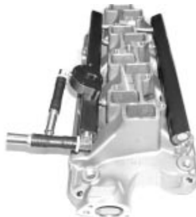
Steps 20-30. Prepped fuel rails.
