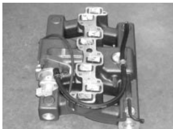
Prepped upper intake.
