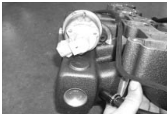
Step 40. Reposition the EGR valve.
