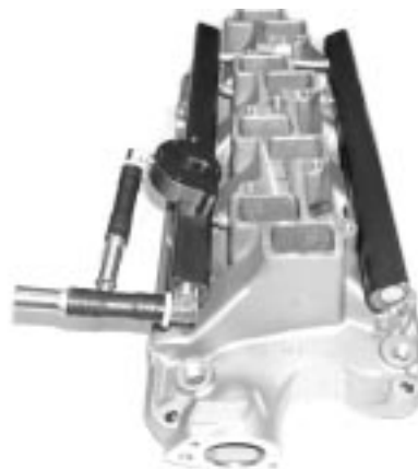
Steps 20-30. Prepped fuel rails.
