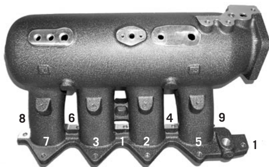
Diagram B TORQUE SEQUENCE
