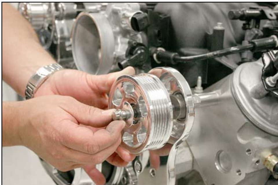
Figure 9: Install Idler Pulleys
