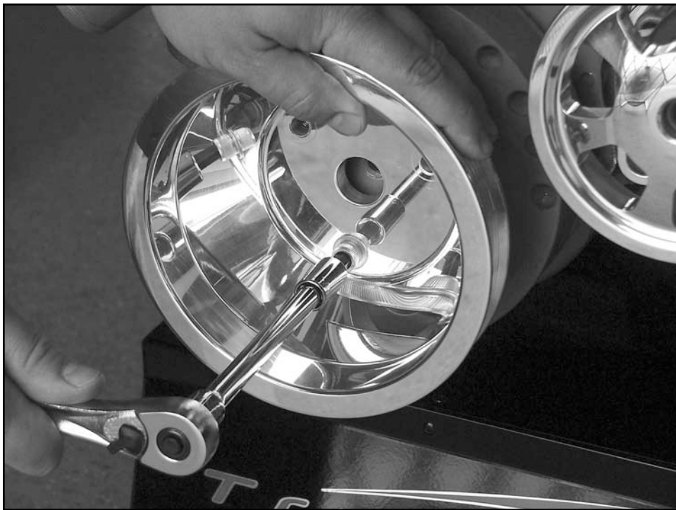
Figure 9: Install Crankshaft Pulley
