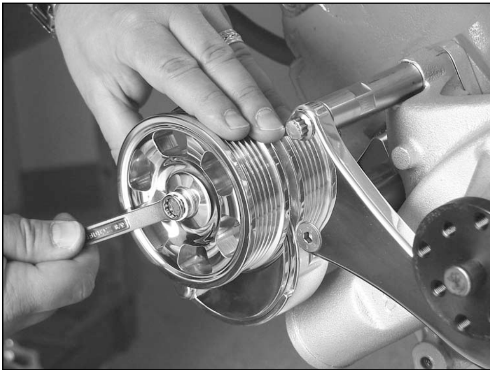
Figure 13: Install Tensioner Pulley
