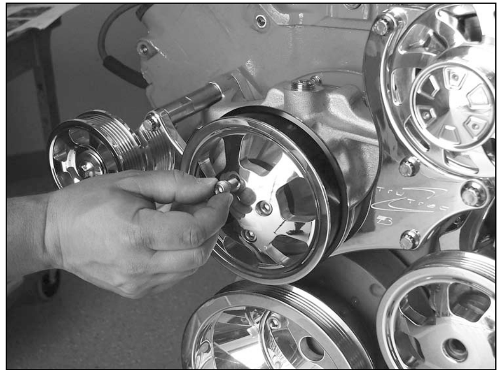
Figure 14: Install Water Pump Pulley onto Pump
