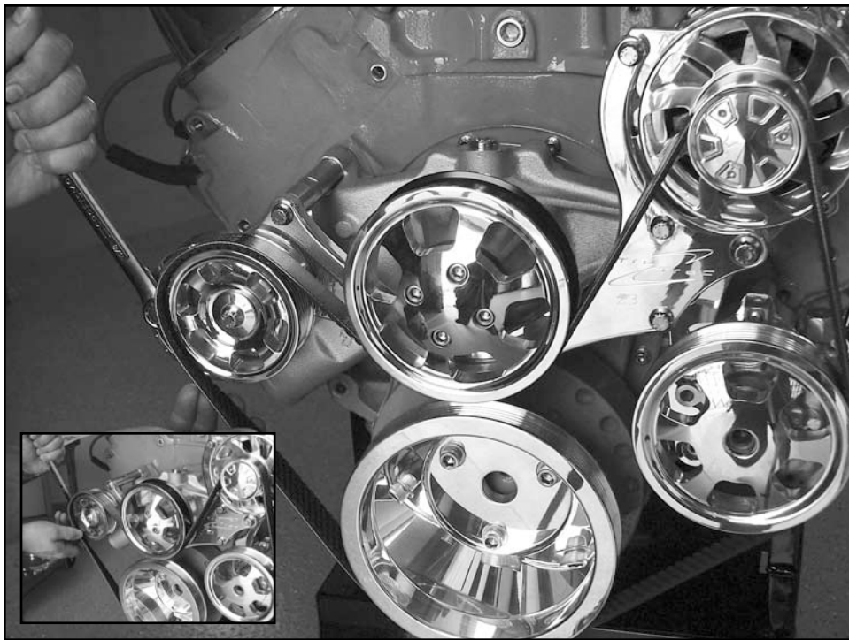
Figure 15: Install Serpentine Belt
