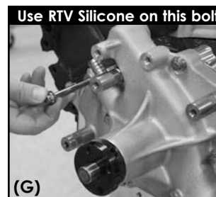
Figure 3b: Install Water Pump
