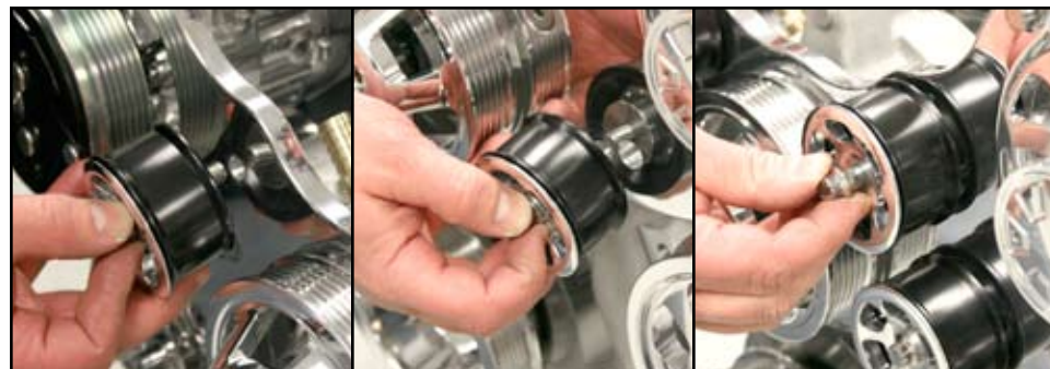
FIGURE 12: Install Idler Pulleys
