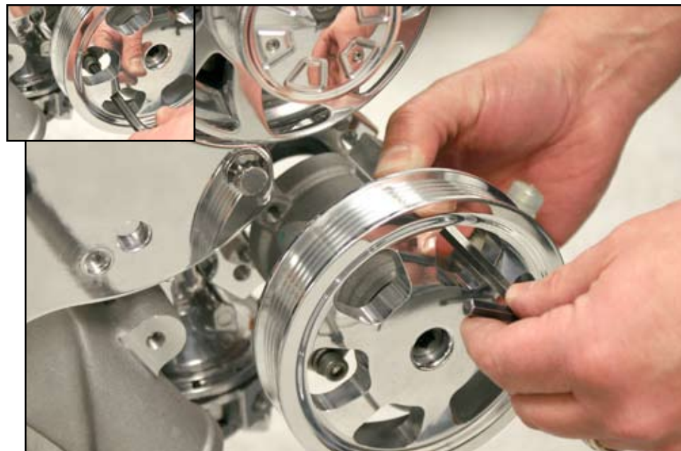
FIGURE 10: Install Power Steering Pump With Pulley
