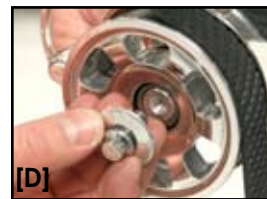
FIGURE 15: Install Tensioner Pulley & Belt
