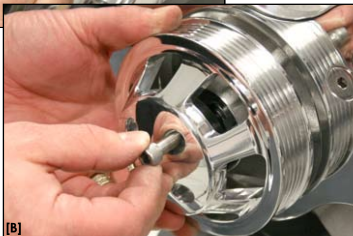
FIGURE 11: Install Crankshaft & Water Pump Pulleys
