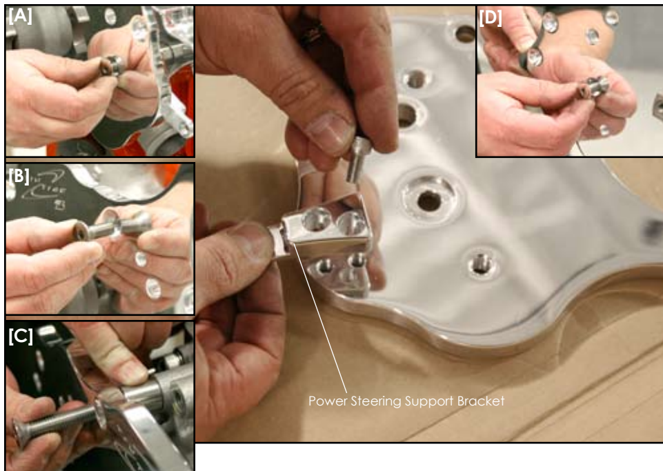
Figure 5 - Install Bridge Bracket
