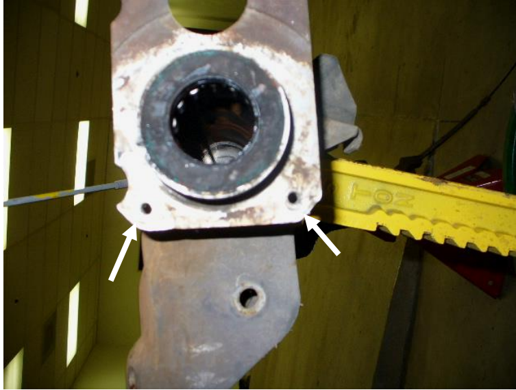
Figure 3: Drill these two holes to .375"
