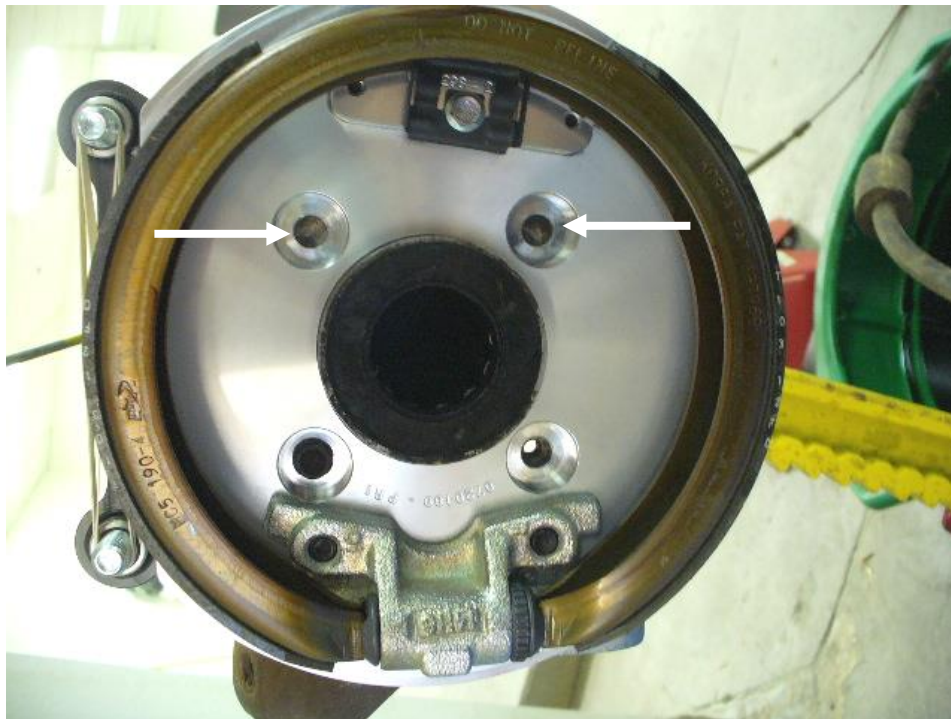
Figure 4: Drill upper two holes to .375"
