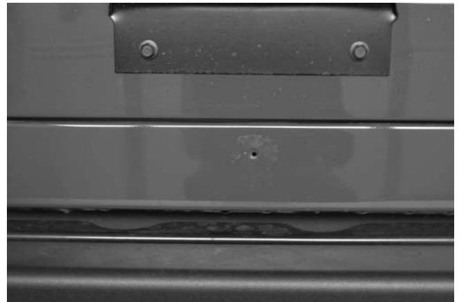
Figure #4 – Remove Tire Stop
