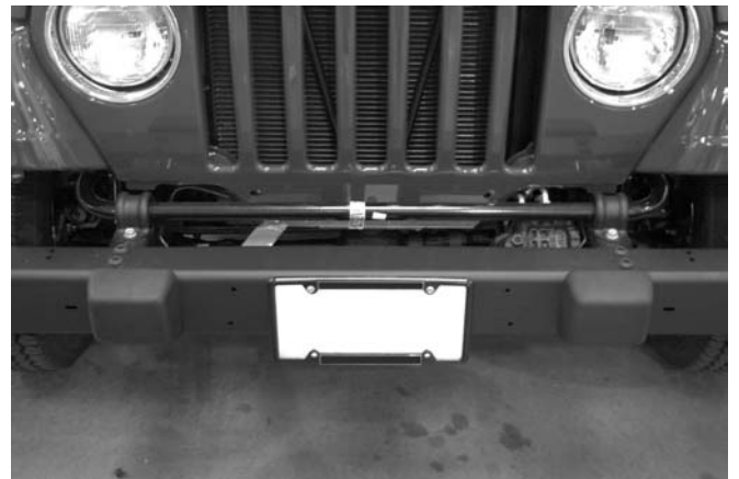
Figure #8 – Factory Front Panel Removed
