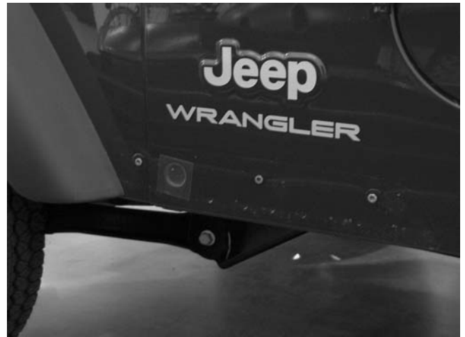
Figure #6 – Remove Stone Guard
