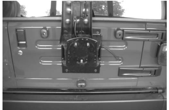
Figure #3 – Remove Spare Tire
