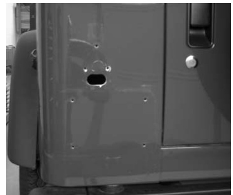
Figure #2 – Remove Tail Light & License Plate
