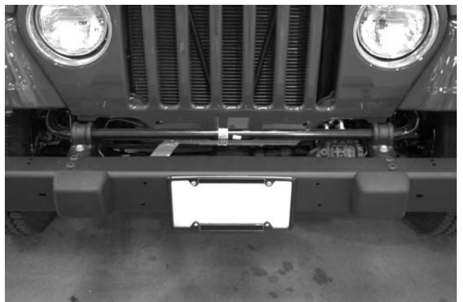
Figure #8 – Factory Front Panel Removed
