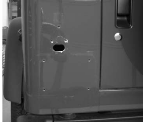
Figure #2 – Remove Tail Light & License Plate
