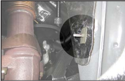
#5 Cut Firewall Bolt
