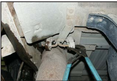
#7 Remove necessary exhaust hangers
