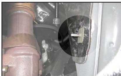
#5 Cut Firewall Bolt
