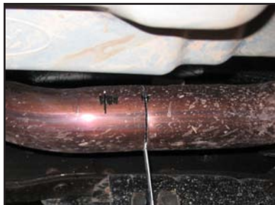
#4 Cut at Bottom of Down Pipe
