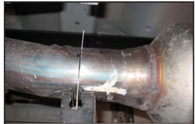
#3 Cut in front of Catalytic Converter
