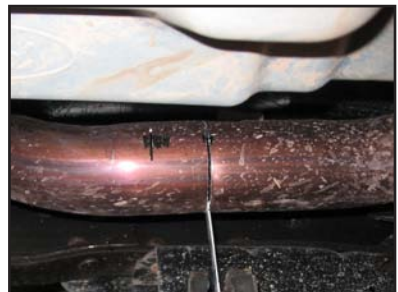
#4 Cut at Bottom of Down Pipe
