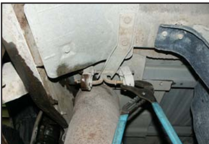
#7 Remove necessary exhaust hangers
