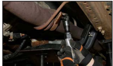
#3 Unbolt flange in front of Cat. Converter
