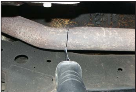
Cut after the bend of the downpipe
