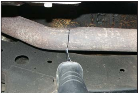
Cut after the bend of the downpipe
