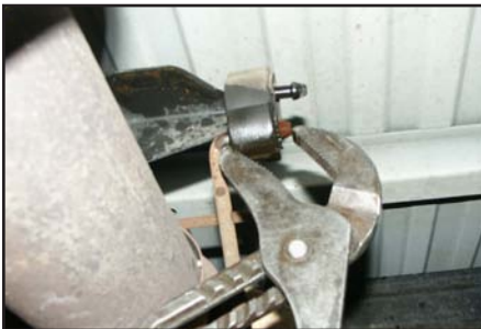
Remove all the necessary exhaust hangers
