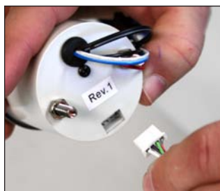
Connecting the Gauge to Conversion Box
