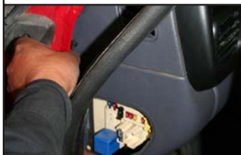
Peel Back Weather Stripping and Remove Sidepanel
