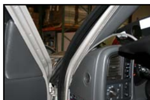
Run wires behind dashboard
