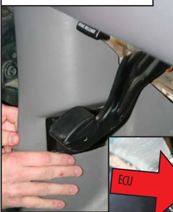
Removal of the Kick Plate
