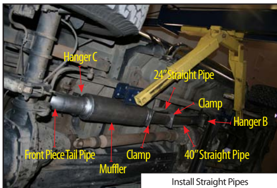
Install Straight Pipes
