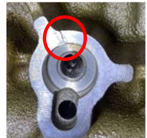
Crack In Mounting Post
