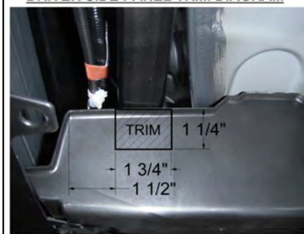
DRIVER SIDE PANEL TRIM DIAGRAM
