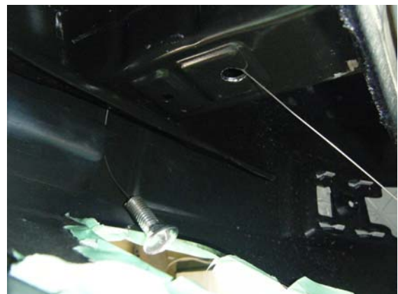
DRIVER SIDE FISHWIRE LOCATION
