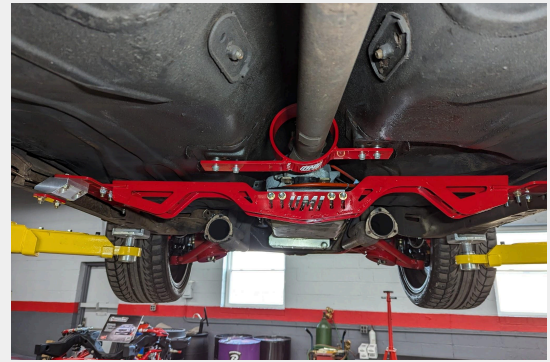
Figure 1: Fully Installed Crossmember
