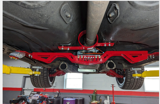
Figure 6: Fully Installed Crossmember
