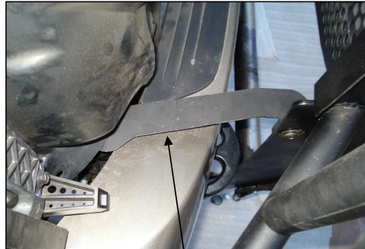
Auxiliary bracket installed, passenger side.
