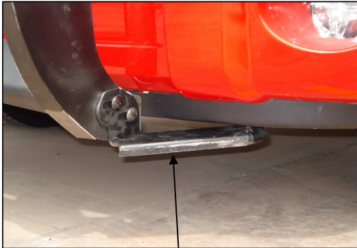
Main bracket installed, driver side.
