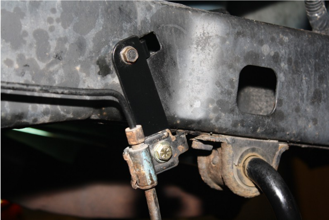
Picture 1 - Driver's Side Rear Brake Line Extension Bracket Shown Installed
