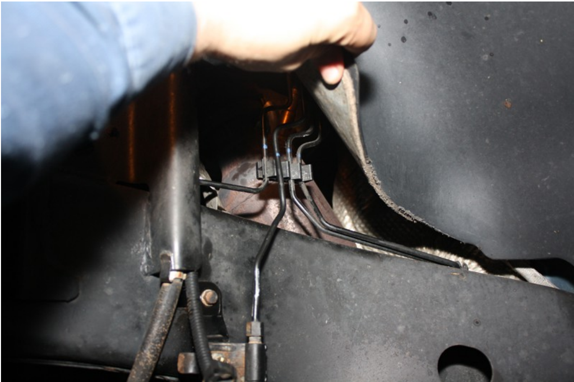
Picture 2 – Driver's Side Brake Line
