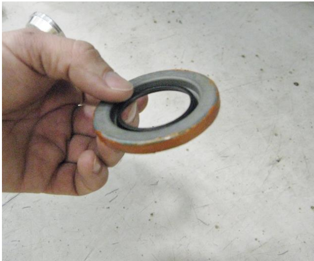
Figure 1 – Use RTV on the Axle Seals
