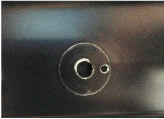
Figure 5 – Drill Anti-Rotation Hole
