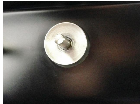
Figure 7 – Thread Bezel onto Switch
