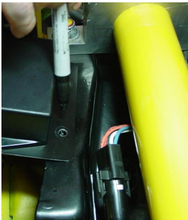
Figure 12 – Locate the Bolt Holes
