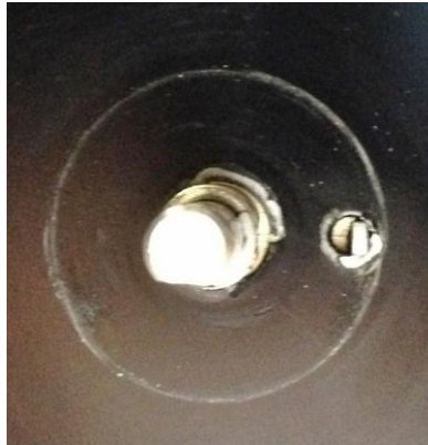
Figure 6 – Install Wiper Switch
