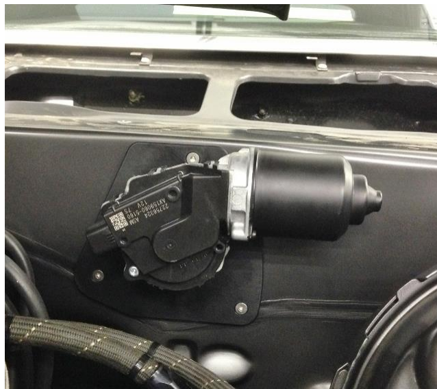
Figure 1 – Attach Wiper Motor to Firewall
