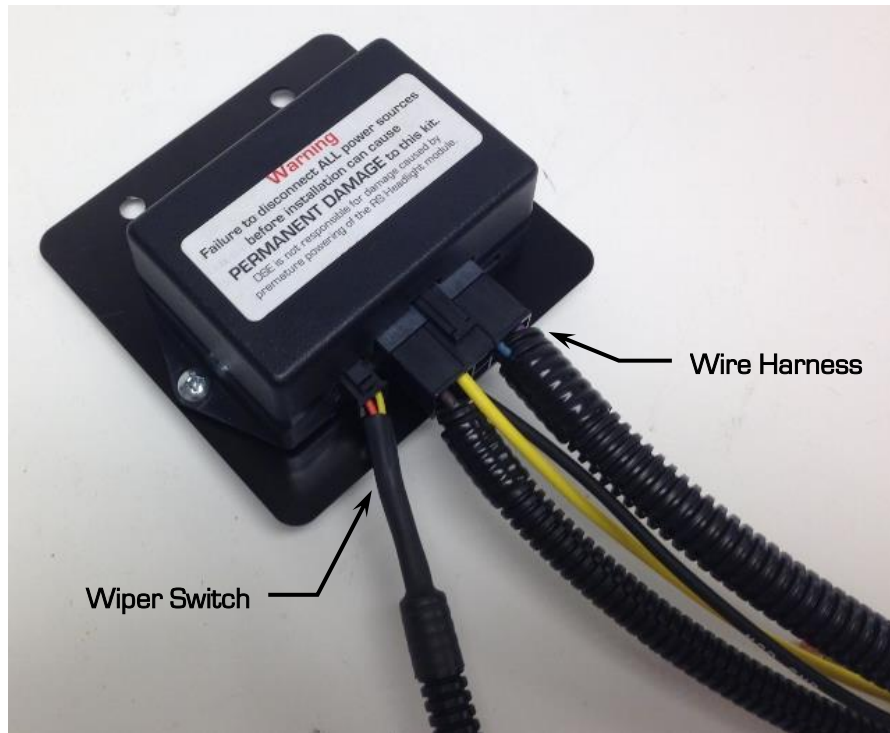
Figure 8 – Connect Wiper Switch & Harness to Module
