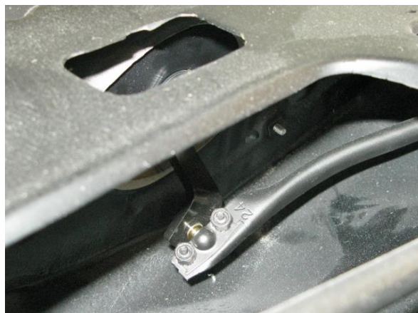
Figure 2 – Attach Pitman Arm to Wiper Linkage
