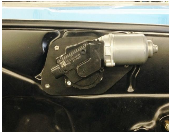
Figure 1 – Attach Wiper Motor to Firewall
