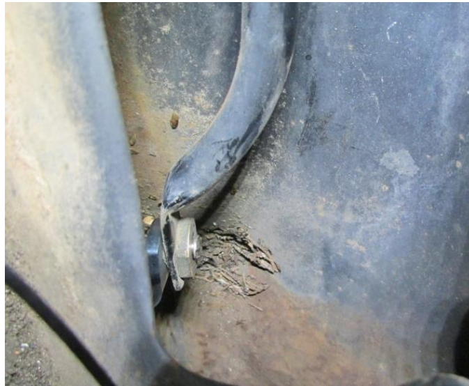
Figure 15 – Install Wiper Linkage to Pitman Arm
