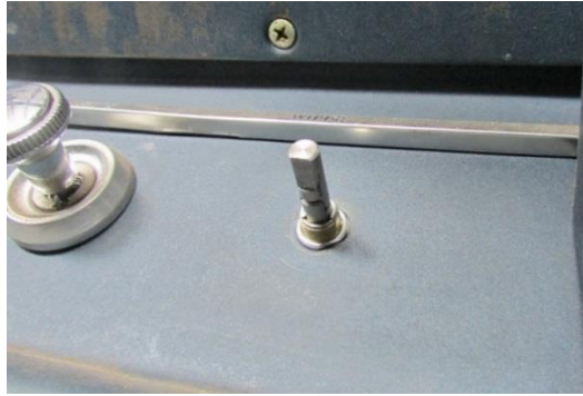
Figure 5 – Install Detroit Speed Switch
