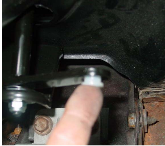
Figure 11 – Installing Bushing in Pitman Arm
