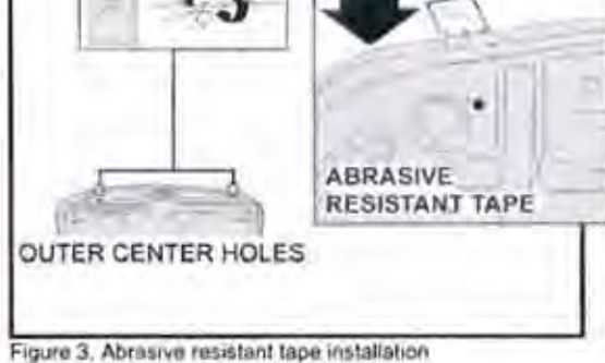
Figure 3. Abrasive resistant tape installation
