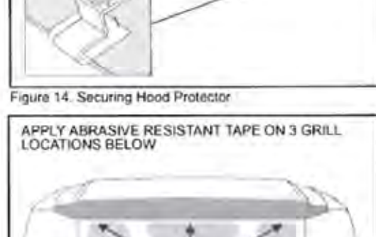
Figure 15. Abrasive resistant tape installation
