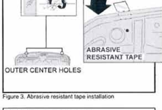
Figure 3. Abrasive resistant tape installation
