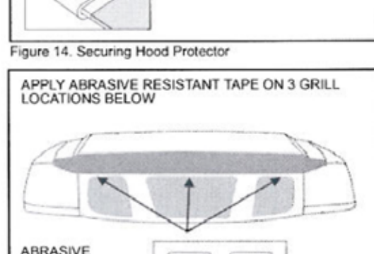
Figure 15. Abrasive resistant tape installation
