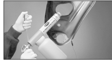
Hold the Powder Gun at various positions and angles to get the best application of powder over the entire part
