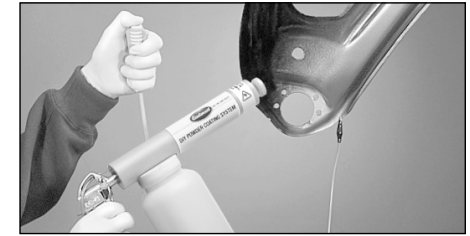
Hold the Powder Gun at various positions and angles to get the best application of powder over the entire part
