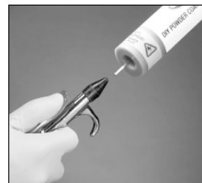
Direct air down nozzle to remove powder
