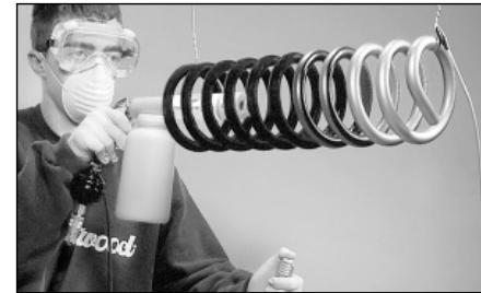
Hold the Powder Gun at various positions and angles to get the best application of powder over the entire part
