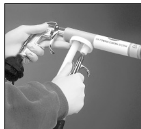
Blow remaining powder out of pick-up tube
